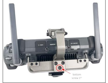
Now, your **LifThor RC PRO PLUS** mount is properly installed. To access the DJI RC PRO PLUS battery bay there is no need to unmount it. The LifThor mount is cleverly designed for you to fold backwards the controller to access the batteries as shown in the pictures.
